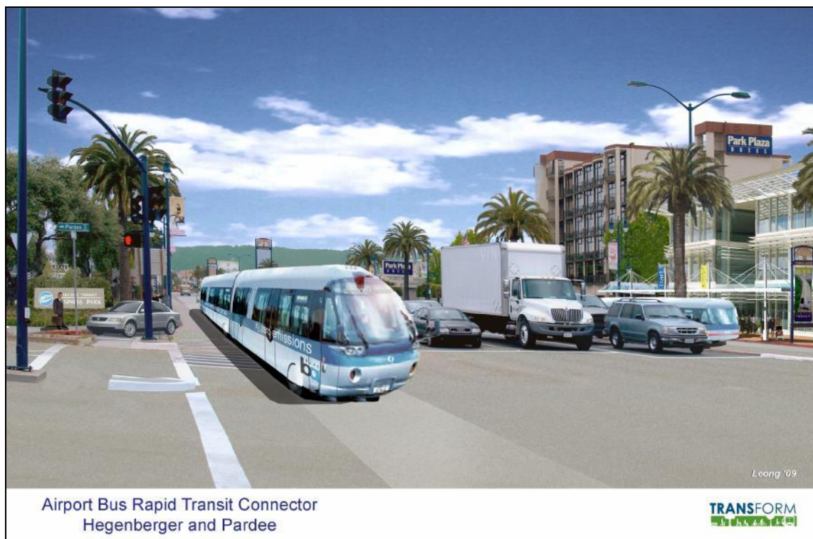
Figure 2 – Right-hand queue jump lanes would allow RapidBART to bypass traffic congestion, greatly improving speed and reliability. New stop is visible across intersection
